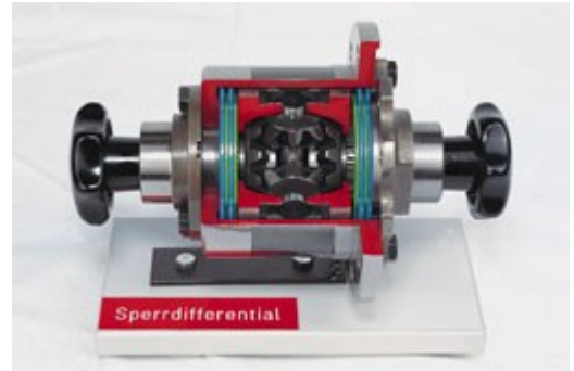
Order No. 1046 Limited-slip differential with multi-disk clutches (ZF)
