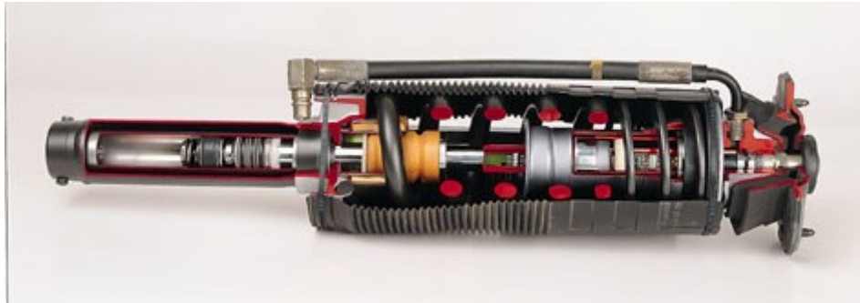
Order No. 1275 Cutaway model: ABC (active body control) suspension strut
