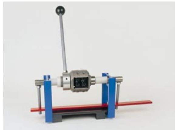
Order No. 1286 Measurement device to measure the locking figure of differentials
