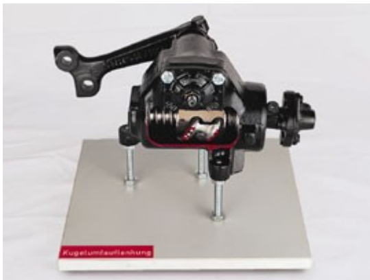
Order No. 1050 Recirculating-ball steering (ball-and-nut steering gear)
