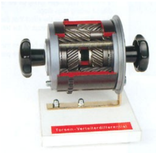
Order No. 1272 Cutaway model: Torsen intermediate axle differential
