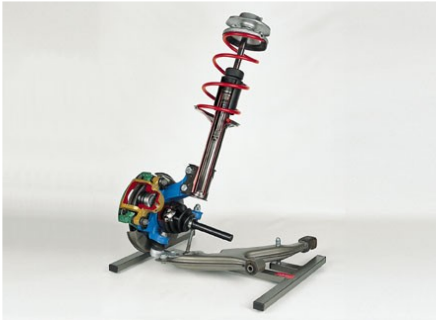
Order No. 1202 Complete suspension strut with wishbone, drive shaft, disk brake with brake disk
