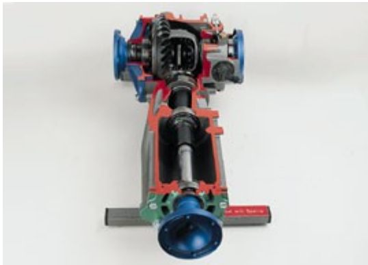
Order No. 1129 Differential with mechanical lock
