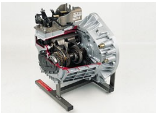
Order No. 1199 Modern five-speed front transmission with differential
